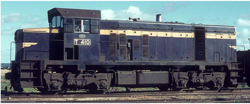
T410 note the sight glass above the handbrake. Courtesy Peter Vincent
